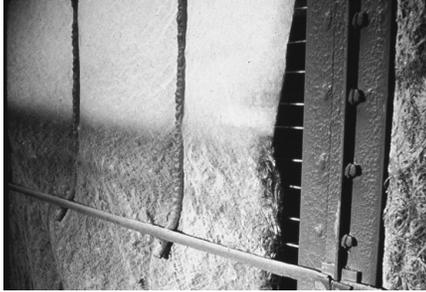
Competitive roll with low tensile strength causes the media to "neck" and pull out of the side channels. Unfiltered air is allowed to bypass the media.
