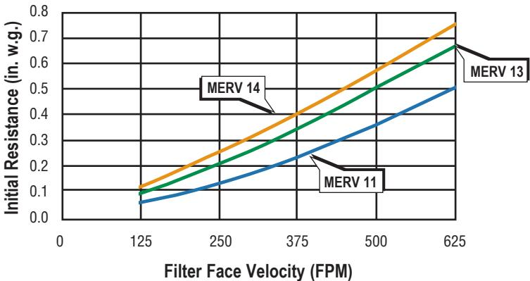
Filters are rated at 500 FPM filter face velocity. Recommended final resistance for all VariCel M-Pak filters is 1.5" w.g.
