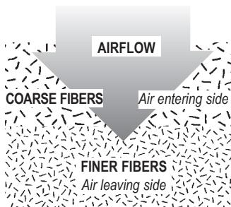
The VariCel M-Pak media pack is constructed with wet-laid fiberglass that is moisture resistant. The VariCel M-Pak filter can withstand exposure to free moisture in the atmosphere, making it ideal for installation in applications where moisture is an issue. The media is manufactured with two layers of glass fibers: coarser fibers on the air-entering side and finer fibers on the air-leaving side. The media pack is bonded to the cell sides using urethane sealant.
